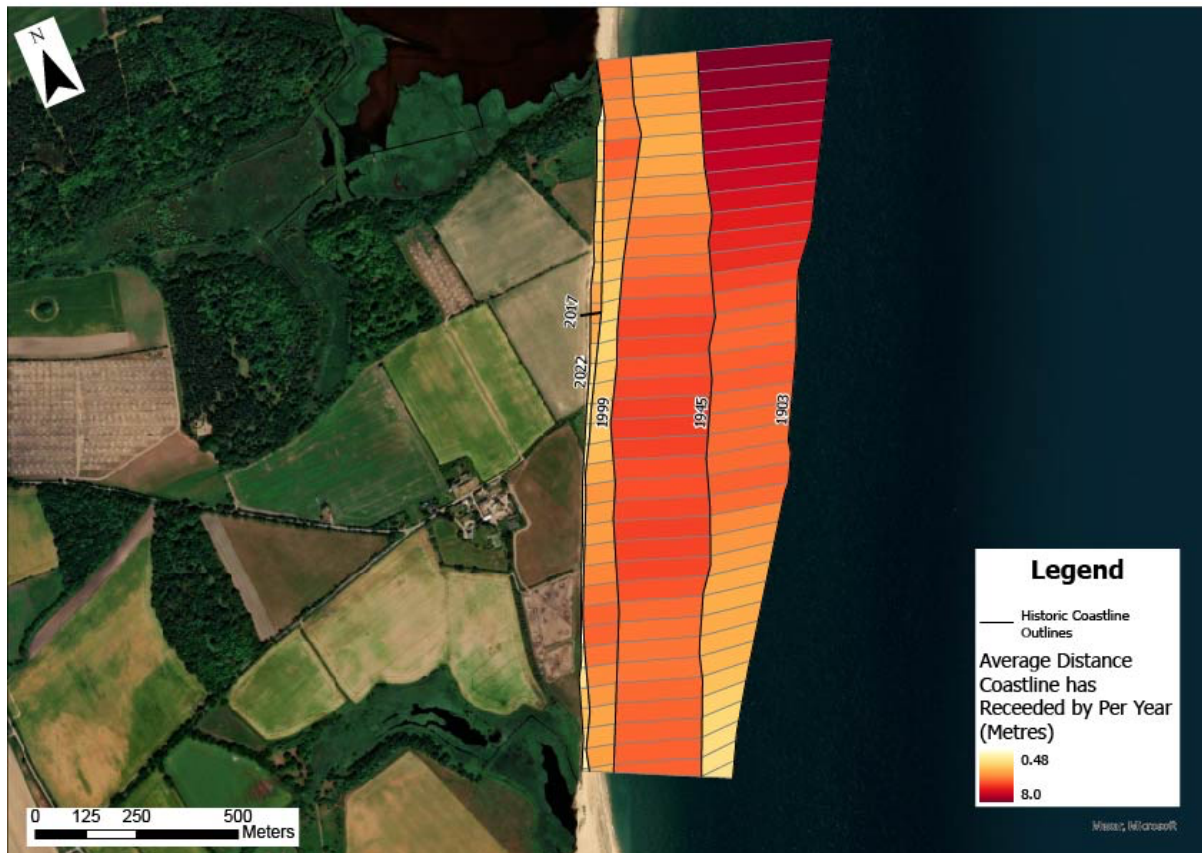
Figure 8 - Historic recession rates at Covehithe between 1903 and 2022. Produced using Esri ArcGIS Pro (2024), using data from Ordnance Survey (1899) and Google Earth (2024).
